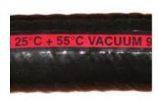
A thermoplastic hose made with a compound of PVC, PU and Nitrile rubber. Black, smooth tube and cover. Flexible, strong, abrasion resistant. Polyester yarn and embedded galvanized steel spiral. Recommended for handling hydraulic oil, fuels, blue diesel, urea (ISO 22241). Abrasion resistant in accordance to ISO 4649: < 90mm³. Temperature range: -25°C to +55°C.
